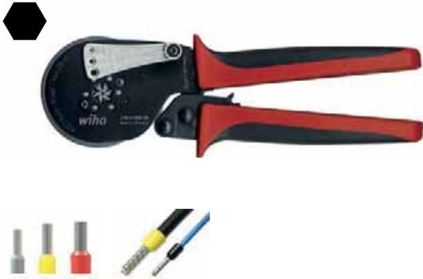
**Increases your efficiency:** Automatic adjustment of wire-end sleeve size with suitable crimping force for a large coverage area of 0.08-16mm<sup>2</sup>. **Makes handling easier:** Thanks to hexagonal crimping, small wire-end sleeves no longer get caught. **Lowers your costs:** An integrated lever enables users to interrupt the crimping process at any time to protect the pliers. **Increases your safety:** Safe work through feed aid prevents crimping the plastic cover of wire-end sleeves.
