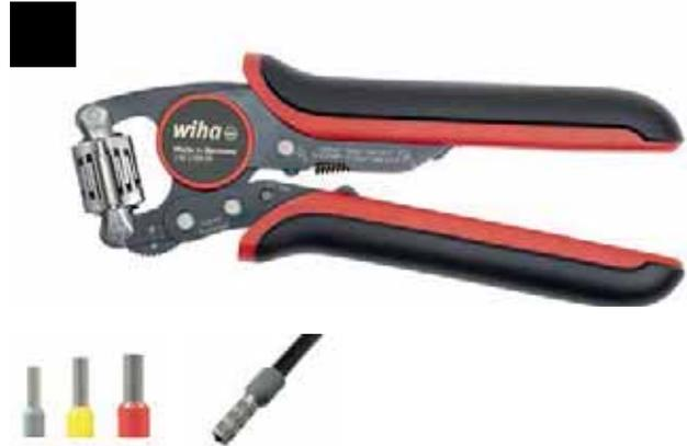
**Makes handling easier:** 360° rotatable crimping die open on both sides for optimal accessibility. **Increases your efficiency:** Automatic adjustment to the wire-end sleeve size with suitable crimping force for a large application area of 0.08 - 16 mm<sup>2</sup>. **Lowers your costs:** An emergency lever enables users to manually interrupt the crimping process at any time to protect the pliers.
